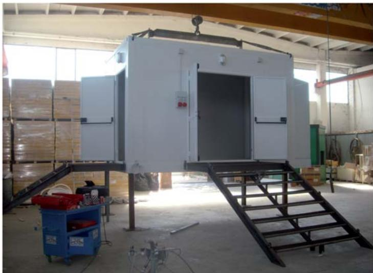
Total length: 4,3 mt - Total wide: 2,5 mt - Total height: 3 mt - Max on load weight: 10.000 Kg
